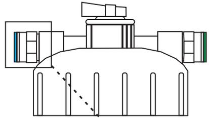
The EZ-FLO system uses push connect fittings to connect the clear and black 1/4" tubing to the cap.
