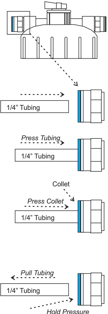
The EZ-FLO system uses push connect fittings to connect the clear and black 1/4" tubing to the cap.
